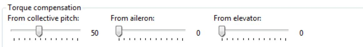
If the main rotor blades change the angle of attack, for example as a result of collective or cyclic commands, the torque, which has to be compensated by the tail, changes too. This could lead to unwanted swings of the tail.
