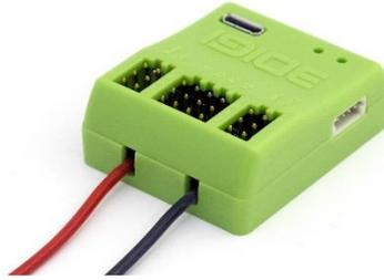
The 3Digi HC variant (HC = high current) has 2 additional cable for direct connection of the external power. These cables have a sufficiently large cross section so that there is almost no loss of voltage between BEC and 3Digi even with power-hungry servos. The cables can be fitted out with various plugs or sockets. We recommend, for example, 2mm or 3,5mm gold contact plugs.
