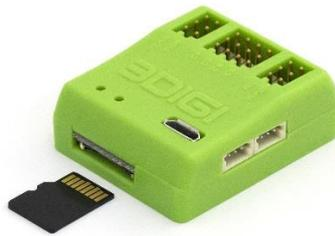
On the back is the slot for the SD card. This should be inserted into the slot with the contacts on the card facing upwards. Then push it in until it stops. The card snaps in then. The card is removed by again pressing it in and will then get unlocked. The card can then be removed by simply pulling it out.
