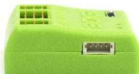
On the remaining side from 3Digi is the special port. This is very flexible usable. You could connect e.g. an external Bluetooth or a GPS module here. More information about the assignment of the socket and voltage levels can be found in the chapter **Connections**.
