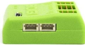
On the side of the 3Digi there are ports for one or two Spektrum satellite receiver. The device connected to the left socket is bound as the master during binding. If an optional satellite is connected to the right socket, this is bound as a slave.
